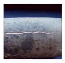
**Lead.** If a scratch test produces a shiny silver color, your pipe is likely made of lead. If you try to attach the magnet to the pipe and it does not stick, you may have a lead pipe.
